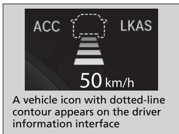
Your vehicle maintains the set speed without having to keep your foot on the brake or accelerator pedal. If there previously was a vehicle detected ahead that kept your vehicle from travelling at the set speed, ACC with LSF accelerates your vehicle to the set speed, and then maintains it.
