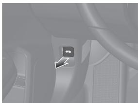
**2** Locate the bonnet latch lever, pull it up, and then raise the bonnet. Once you have raised the bonnet slightly, you can release the lever.
