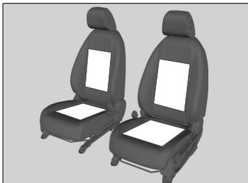
The ignition switch must be in ON
