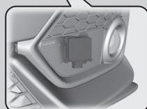
The radar sensor is in the lower bumper next to the fog light\*.
