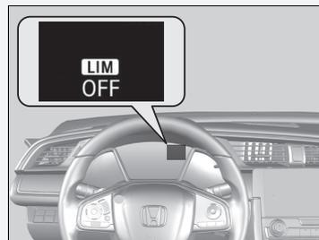
If there is a problem with the system when you are using the adjustable speed limiter, the beeper sounds and **OFF** comes on. The adjustable speed limiter will be turned off.
